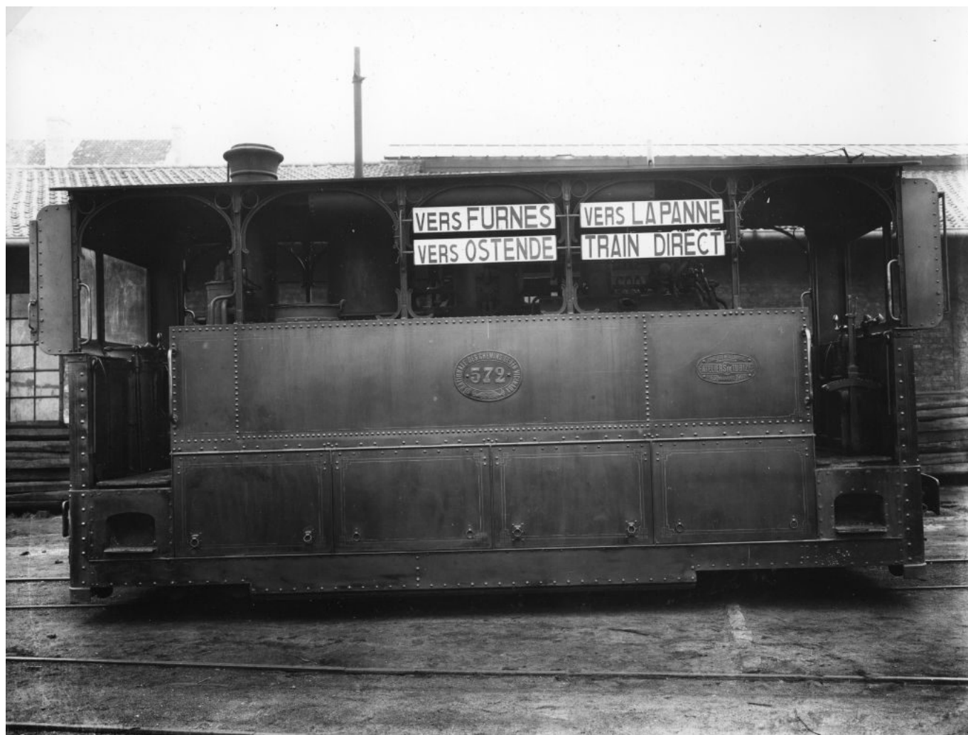
Tz 1650 - Tubize type 16 - SNCV 572 type 16 (Coll. M. Hennequin, photo SNCV, Archives PFT)
